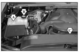
If the coolant inside the coolant surge tank is boiling, don't do anything else until it cools down. The vehicle should be parked on a level surface.
